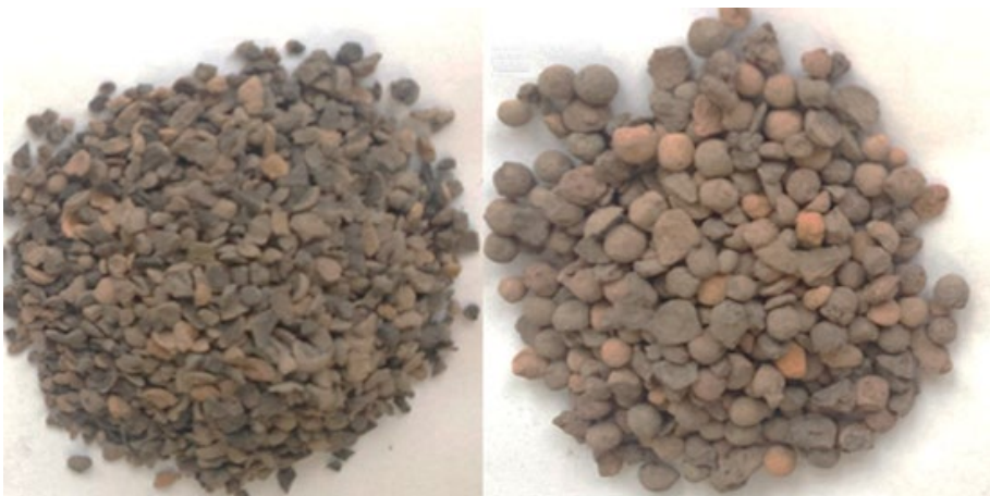
Figure 4. Certyd aggregate with a grain diameter of 2-4 mm and 4-8 mm
