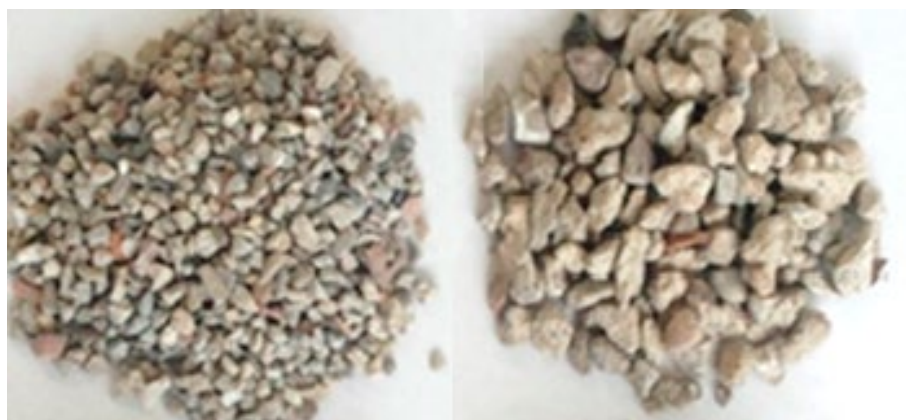
Figure 5. Aggregate from concrete recycling
