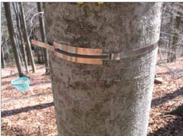
Figure 2. Beech tree at Coll de Te with dendrometers
