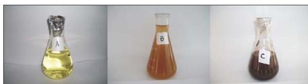
Figure 1. Optical photograph of (A) \text{AuCl}_4 solution (B) Fruit extract (C) Fruit extract + \text{AuCl}_4
