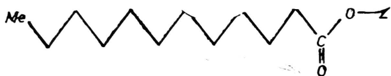
Fig. 4. Salts of long chain carboxylic acids. Tensides or initial stages for tensides
