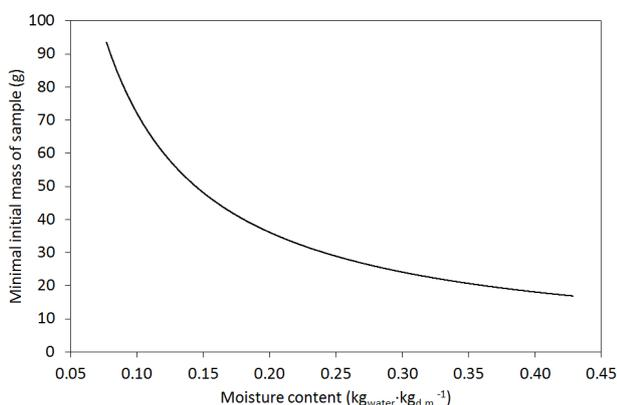
**Fig. 1.** The relation between the minimal initial mass of a sample and the moisture content of kernels ( $\delta_z=0.2\%$ ,  $M_0=0.43 \text{ kg}_{\text{water}} \text{ kg}_{\text{d.m.}}^{-1}$ ).
