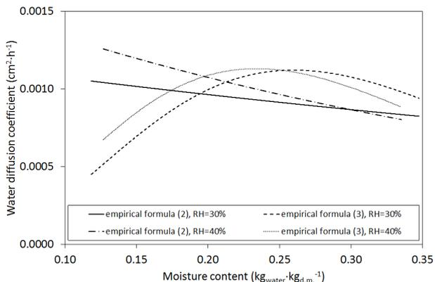
**Fig. 3.** The relation between the water diffusion coefficient and the moisture content inside corn kernels obtained for the drying air temperature of 40°C and the relative humidity of 30 and 40%.
