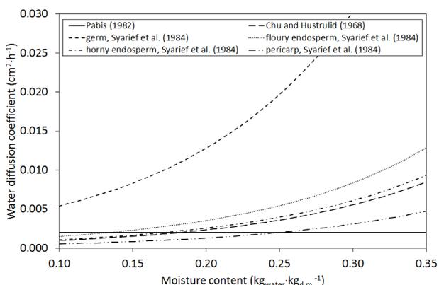
**Fig. 4.** The relation between the water diffusion coefficient and the moisture content inside corn kernels for the drying air temperature of 40°C, simulations based on the literature data for the water diffusion coefficient.
