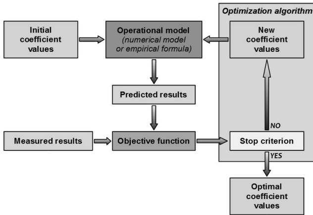
**Fig. 2.** The diagram of the identification algorithm.
