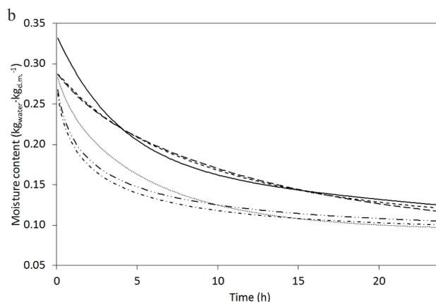
**Fig. 5.** Generalized experimental data and the predicted values of the moisture content inside corn kernels dried in a thin layer at the drying air temperature of 40°C and the relative humidity of: a – 30 and b – 40%.
