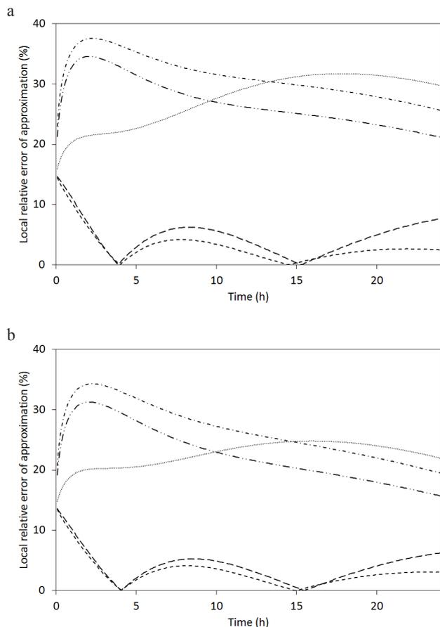
**Fig. 6.** The local relative error of approximation for predicting the moisture content inside corn kernels dried in a thin layer at the drying air temperature of 40°C and the relative humidity of: a – 30 and b – 40% for 5 simulation variants. Explanations as on Fig. 5.
