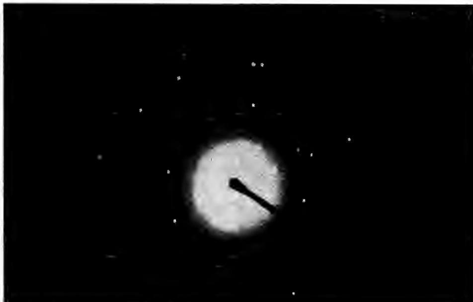
Fig.6. The electronic diffraction on starch crystal shown in Fig.5
