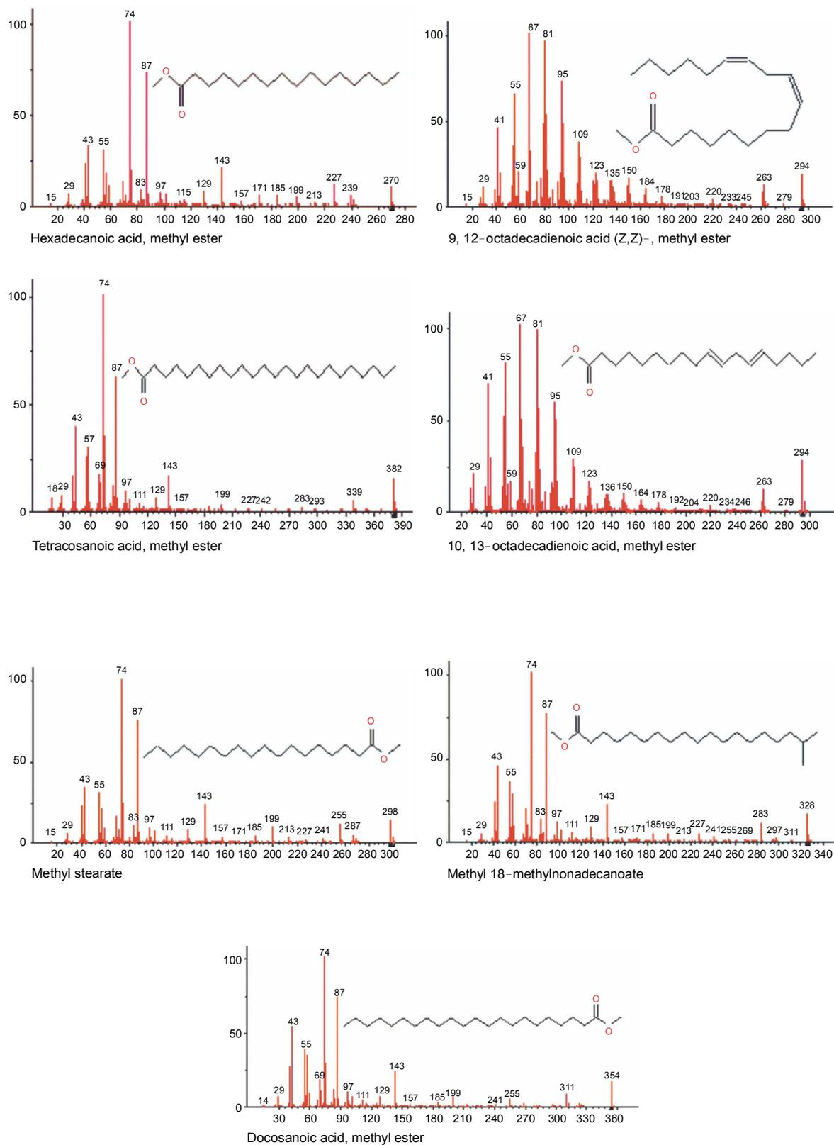
**Fig. 3.** Spectra and structures of some compounds identified in CO extracted by the cold method
