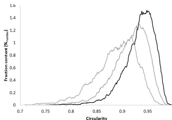
Fig. 3. Distribution of circularity of the investigated sands obtained by the image analysis from the optical microscope. Explanations as in Fig. 2.
