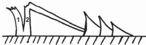
FIGURE 3. Breakage split at butt end
