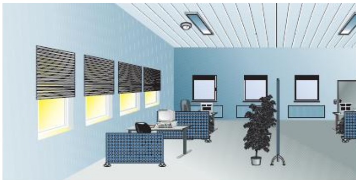
Fig. 6. Principle of indoor artificial lighting control depending on varying natural light conditions [1]
