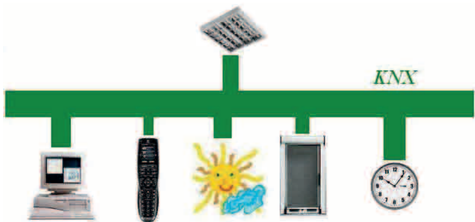
Fig. 1. Lighting control opportunities in KNX/EIB system.
