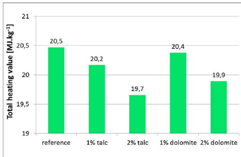
Fig. 4 Effect of additives on total heating value of produced wood pellets
