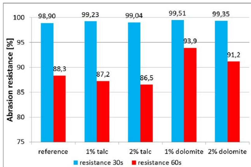
Fig. 2 Effect of additives on abrasion resistance of produced wood pellets
