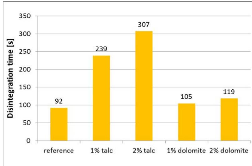
Fig. 3 Effect of additives on disintegration time of produced wood pellets in water test
