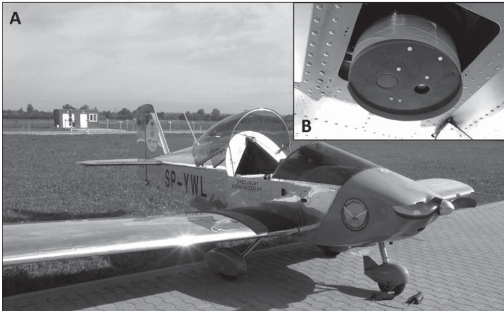
FIGURE 2. Modernized aircraft LSA class (A) and container with photo camera on the hanger under the fuselage (B)
